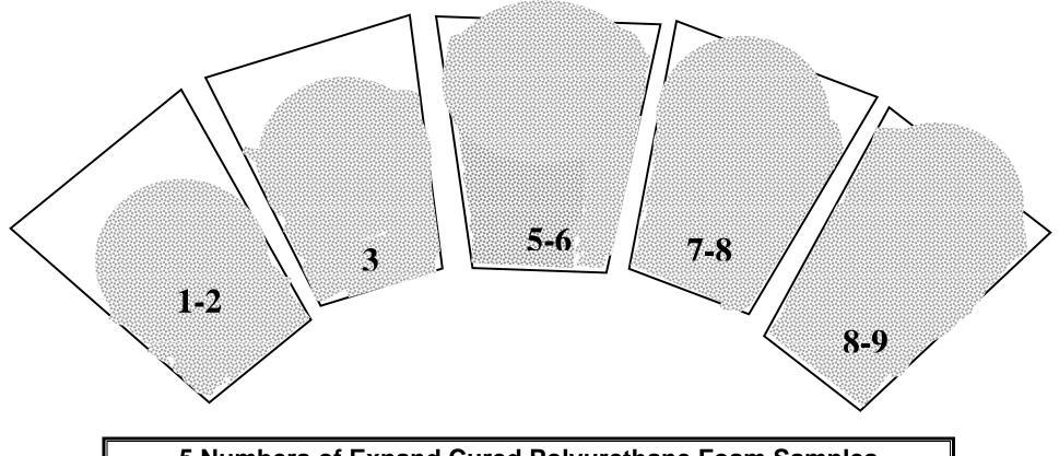
5 Numbers of Expand Cured Polyurethane Foam Samples "LaMaCo-Inject Seal Elastic"
